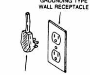
POWER SUPPLY CORD WITH 3-PRONG GROUNDING PLUG
